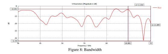
The bandwidth of proposed antenna is 21.877GHz (61.877 GHz – 40 GHz). Therefore total bandwidth is 27.042GHz (5.165GHz + 21.877GHz).
