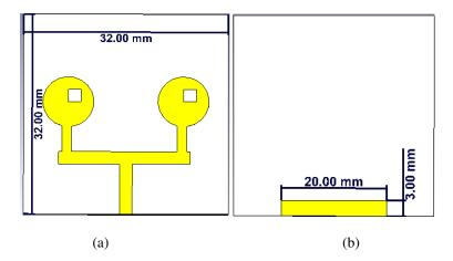
Figure 3: (a) Top view (b) Defected Ground Sturcture
